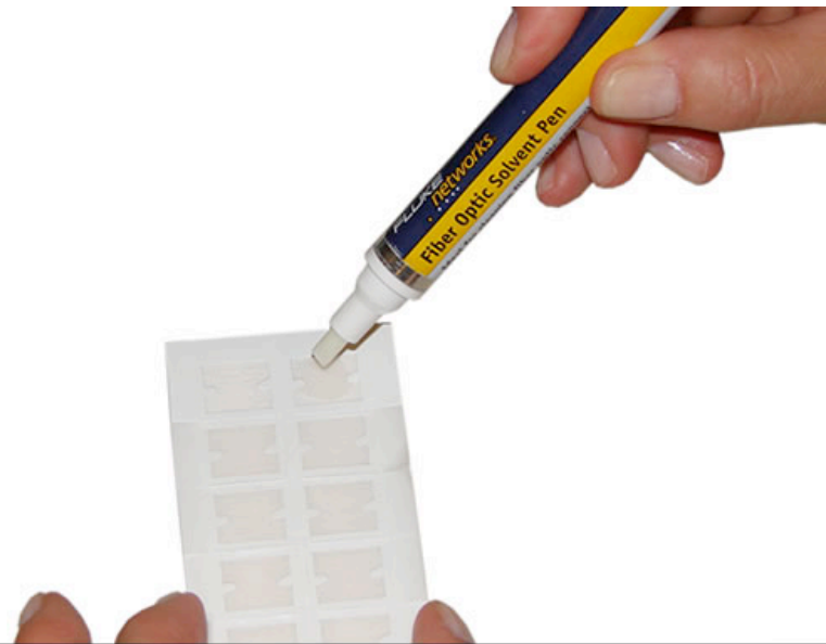
Using the Fiber Optic Solvent Pen, dab a small amount of solvent onto the pad.
