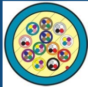
Reduced O.D. 48F Loose Tube Cable (0.231")
